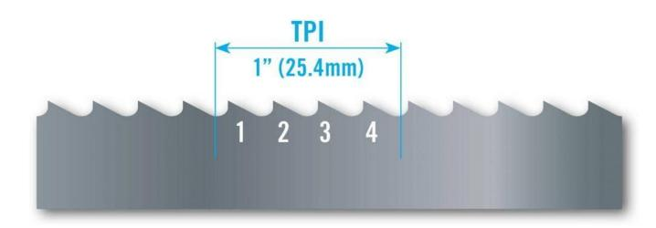
The number of TPI defines the pitch of the blade and can vary from 1 to 32 TPI. On some bandsaw blades there are different pitches on the same blade referred to as Vari-Pitch. TPI is measured from gullet to gullet, not tooth tip to tooth tip – this is known as pitch.
